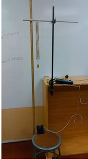
Figure 1. A set up of a single mass (bob)-spring system. You can see the motion detector sitting on the stool in the photograph. Here, the bob has a mass of 200 grams, but the spring constant is unknown.
