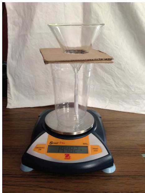
Figure 1. Shown is the apparatus used for collecting data on evaporation when the container was a conical funnel. The bottom of the funnel is sealed and it is supported by cardboard cutout resting on a beaker lip. The apparatus with the Petri dishes was similar, with the Petri dish in place of the beaker and its contents.
