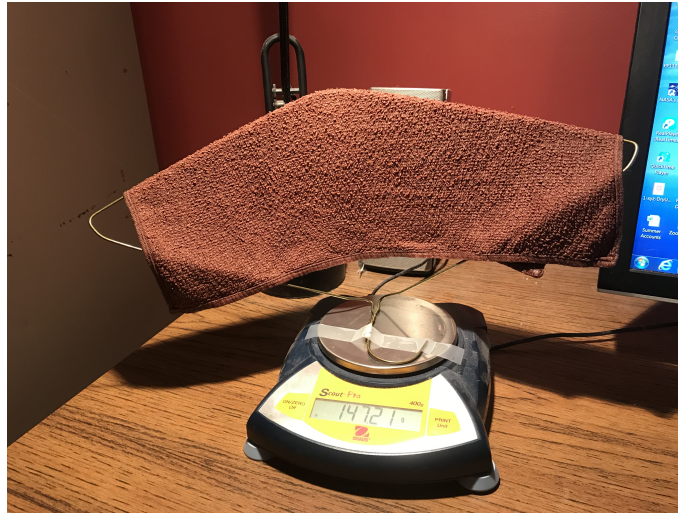
Figure 1. Apparatus used to collect data for drying cloth. Cloth is suspended over wire coat hanger stand taped to an Ohaus Scout Pro scale which is connected to a computer via Vernier Software to record data (mass of configuration in grams) over time. In our case this was every 7 minutes.
