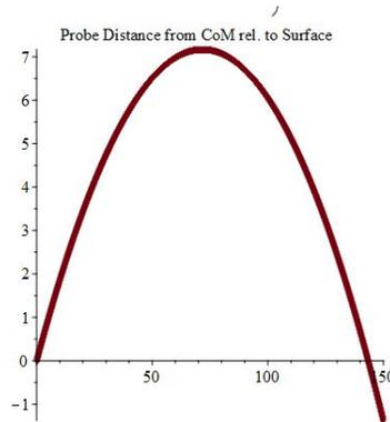
This is semi-parabolic, but has some adjustments. This was found using maple to solve the ODE numerically. I tried several different methods of solving it analytically, but did not get any useful results. This numeric plot is as expected, and as the initial velocity increases the height and time of flight increases, until it is greater than the escape velocity, when the object would leave the orbit entirely.
