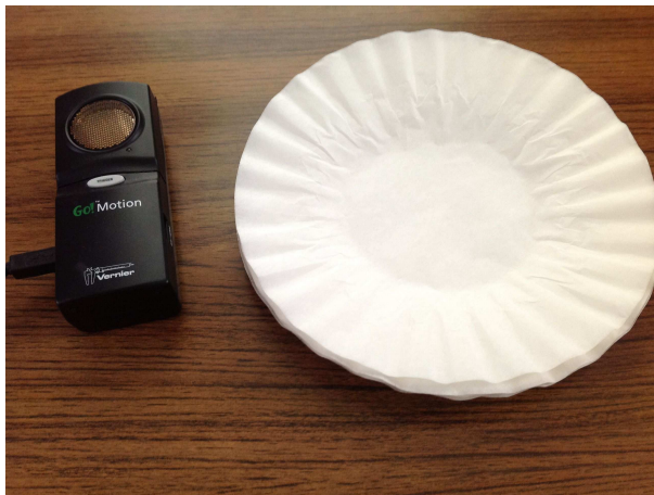
Figure 1. Vernier Software & Technology Motion Detector and stack of coffee filters.
